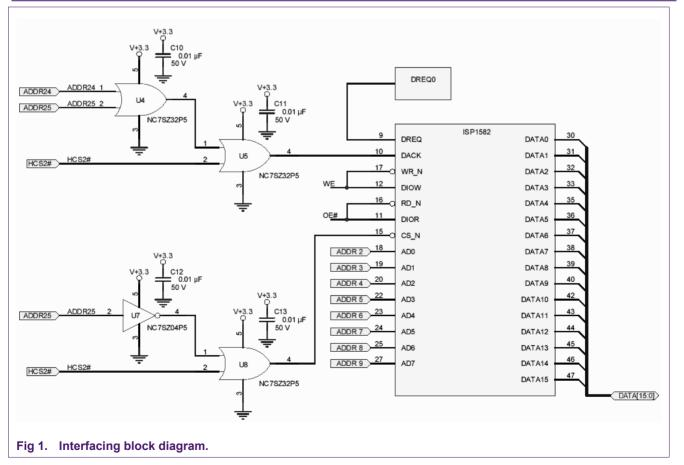
For direct memory access (DMA) to the ISP1582 from the Cotulla chip, the following addresses are used. Using simple logic gates in between Cotulla and the ISP1582 can generate the required DACK signals.
